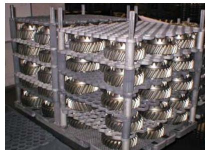
Fig. 3. Even heavy gears can benefit from helium quenching.
